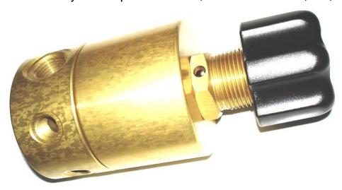
**Application**: For very high continuous flow rates and high differential between the inlet and outlet pressures the regulator may tend to freeze up. For these severe applications two regulators in parallel or some form of heating on the regulator body will usually solve the problem.
